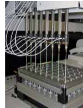
Gas-inducing millilitre-scale bioreactor system with 48 stirred-tank reactors arranged in a bioreaction block (Source: Prof Weuster-Botz, TU München)
