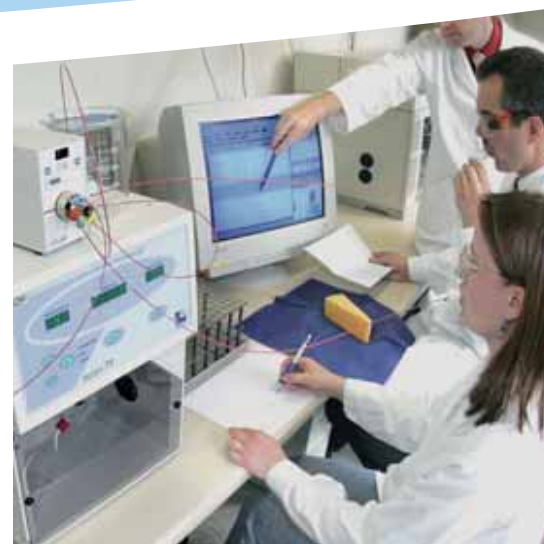
The new high-temperature liquid chromatography method developed by Symrise allows researchers to separate aroma molecules and flavouring components from solutions and thus enables the simultaneous technical detection and human taste evaluation. (Symrise LC-TASTE™ Technology, Courtesy of Symrise)
